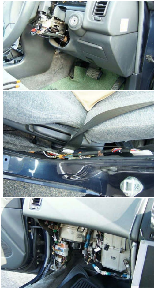
Figure 11. Hand wiring for sensors.
