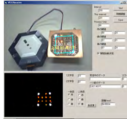
Figure 10. An example of recognition from a LED VCC marker
